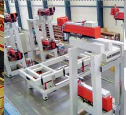
system designed to support measure and reposition the different parts involved at the final assembly position.
