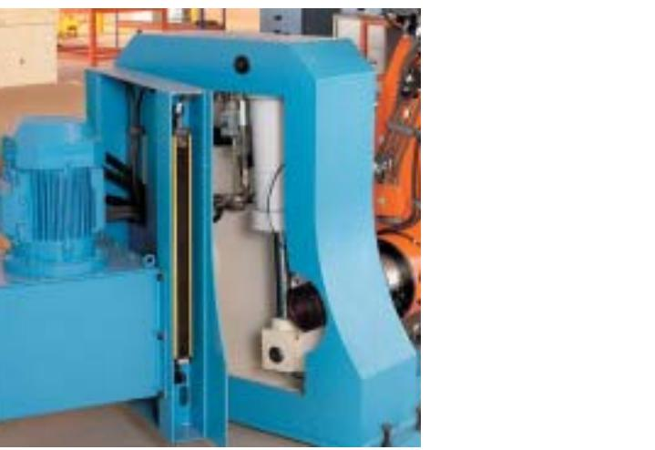
The longitudinal movements of the arms to catch, leave and align the reel can be carried out through hydraulic cylinder that guarantees a perfect operation and balance in the arms.
