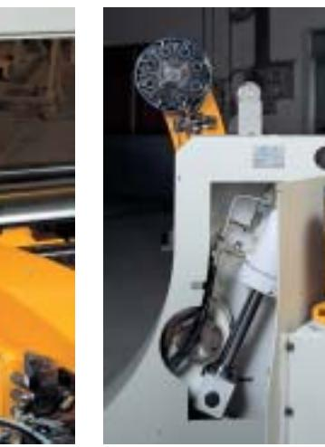
The longitudinal movements of the arms to catch, leave and align the reel can be carried through spindle, by electric motor with a system that limits the axial force when catching the reel.
