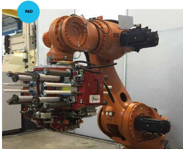
The aim is to create a new AFP platform in a robot for 2D and 3D lamination processes.
