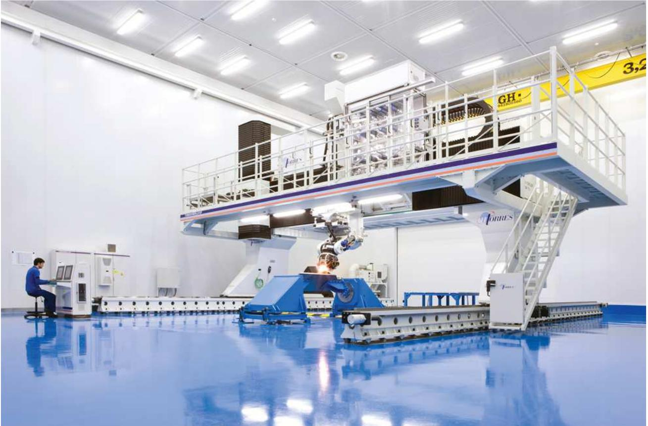
Now, employing AI and machine-learning, an MTorres device can laminate a wing at 4,000 inches per minute while self-detecting flaws in real time; calculating more efficient "routes" among the millions that a machine might follow to make the airplane part; and collecting previously unimaginable amounts of data on every aspect of the job — data continually crunched and fed back into the software, where it is optimized and adapted to the manufacture of other parts of the plane.
