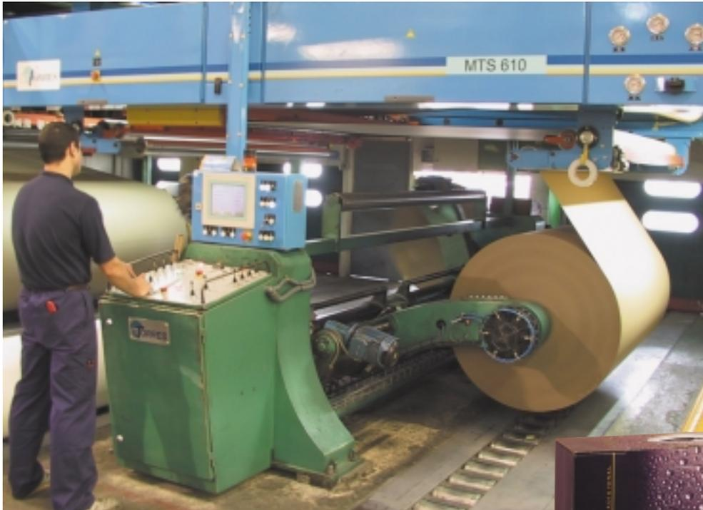
ONE OF THE KEY DEVELOPMENTS OF THIS NEW SPLICER IS ITS ABILITY TO MAINTAIN A CONSTANT WEB TENSION, EVEN DURING ACCELERATION OR DECELERATION DURING THE SPLICE CYCLE.
