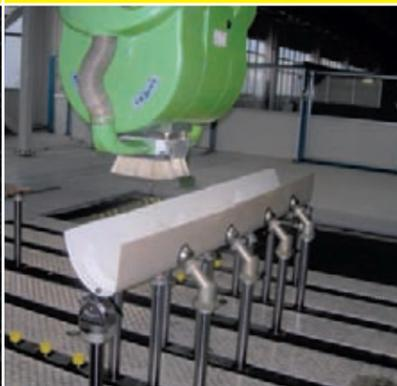
All supports rods move simultaneously in X, Y, Z axes and are automatically locked in their final position. All motions are servo driven and NC controlled. Ground guide ways, rack and pinion and ball crews systems are used to drive the axes.
